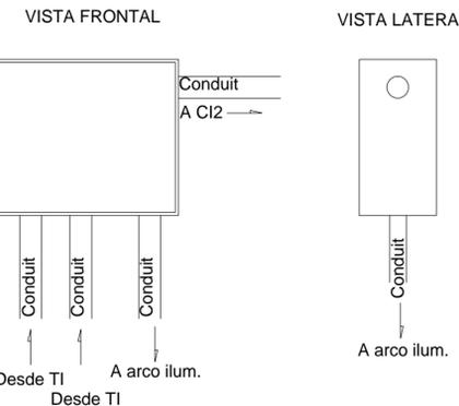
CI.2 A CI.8: CAJA DE PASO Y CONEXION (A DIMENSIONAR) DE ALUMINIO INYECTADO IP65
